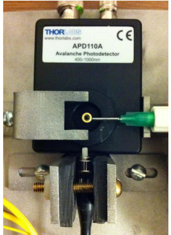
**Figure 3: Close up of sensing area in photodetector**
