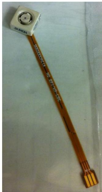
**Figure 5: (Note, there are three pins, but only power and ground were used. The third pin is for speed sensing.**
